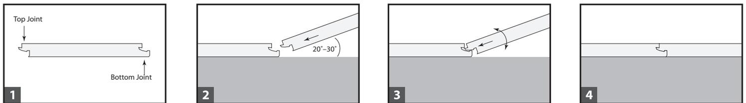
To lock pieces of UniClic® flooring together, lay a piece on the floor with the Bottom Joint facing you (Figure 1). Take another piece, and insert the Top Joint at a 20° – 30° angle (Figure 2). Gently move the piece up and down while exerting forward pressure (Figure 3) until the pieces click into place (Figure 4).
